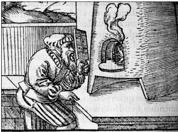
FIGURE 2 A woodcut showing a workman protecting his eyes from the radiant heat of an assay furnace by viewing the white-hot crucible through a narrow slit in a wooden board
