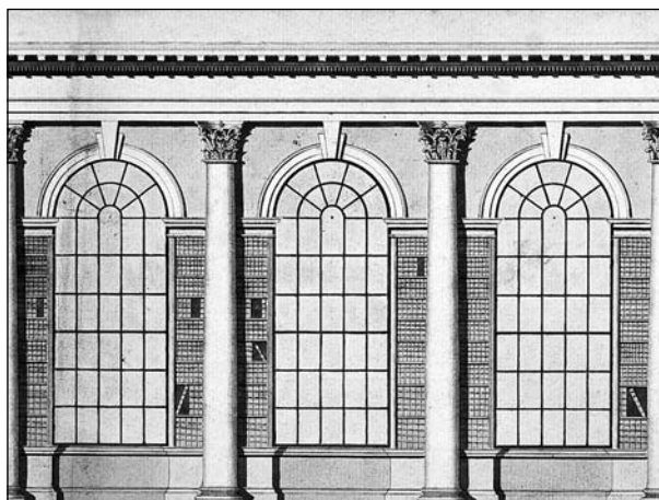
FIGURE 3 A detail of the hall's library windows with their segmented arches, from one of Craig's surviving plans.
